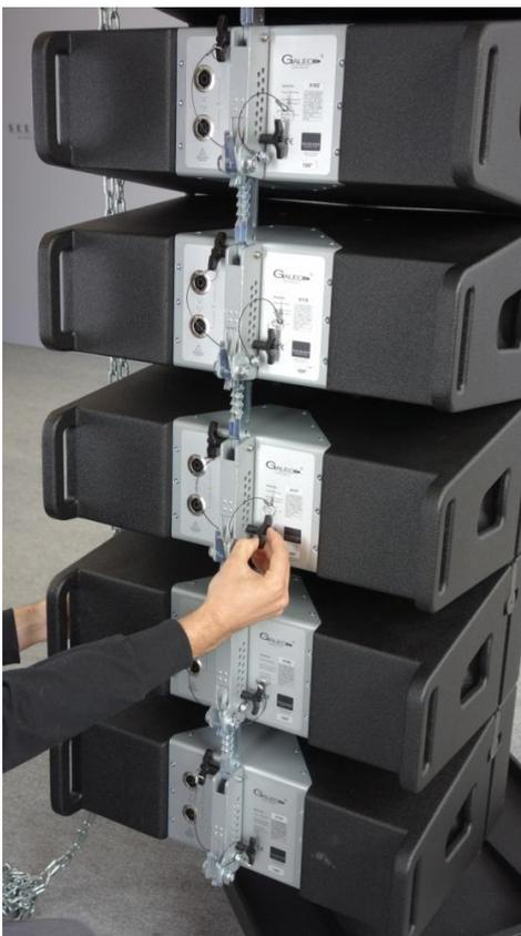
Presetting the desired splay angles in flown, not curved array
