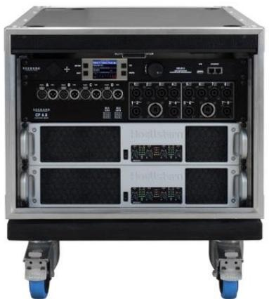
The 7U standard system rack offers 8x inputs (4x analog and AES, 8x DANTE optional) and 8x amplifier outputs for the speakers. The heart of the system is the HDLM 8 system controller, which is responsible for the entire speaker processing. All connections required for the system are located on the front of the CP 4.8. connection panel and can therefore be reached quickly by the user. On the rear of the CP 4.8 there is also the three-phase power distribution with the CEE 16 A connector.
