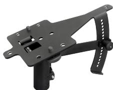
Tilt adapter with adjustable tilt from 0° to 37,5° (2,5° steps), integr. pole mount adapter with clamping device, 2 x knurled screws (M10 x 20 mm), max. load 50 kg
